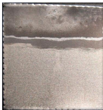
Fig. 3: Aluminium-coated aluminum plate with zinc as intermediate layer
