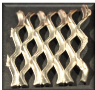
Fig. 4: Aluminium-coated steel wire mesh
