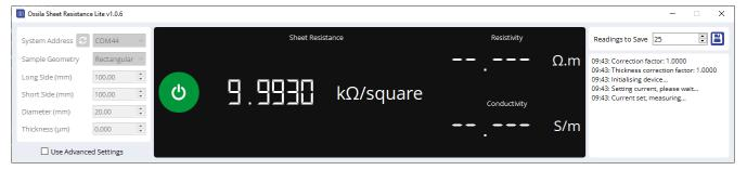
Control your four-point probe with our free, user-friendly Ossila Sheet Resistance Lite software. The software can calculate appropriate geometrical correction factors for the sample geometry and the resistivity and conductivity of the sample to allow for extensive, accurate electrical characterization of materials.
