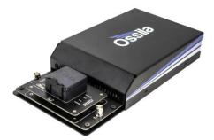
The Ossila LED Measurement System provides a low cost and complete solution for performing current-voltage-luminance (IVL or JVL) characterisation of LEDs. The device holder has built-in light sensors to allow for illuminance, luminance, and white count measurements. To simplify device testing, the software will also calculate the current and power efficiency of your LED. Lifetime mode, meanwhile, measures the performance of the LED over an extended time under a constant voltage.
