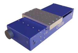
With a 50 mm to 200 mm travel distance and a precision ball screws, Ossila stages offer accurate positioning control. Calibrated according to ISO 230-2:2014 standard with our traceable calibration system.
