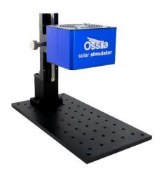
Compact and low price, the Ossila Solar Simulator is ideal for characterizing small-area solar cells, providing:
